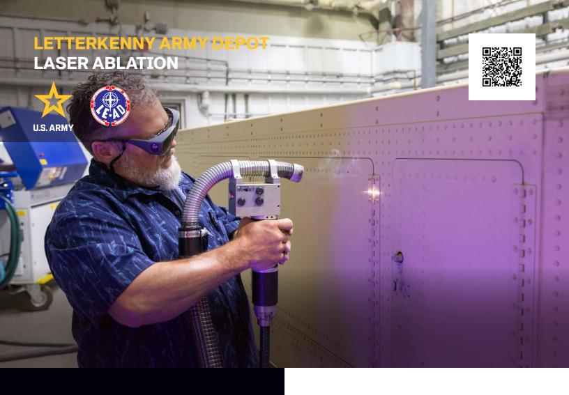
Laser ablation is a subtractive manufacturing technology that utilizes pulsed laser energy to rapidly remove paint and corrosion from solid surfaces by heating and evaporating unwanted materials.
